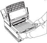
3. Lift the image drum unit out, keeping the image drum unit out of direct sunlight. DO NOT touch the green surface of the drum.
